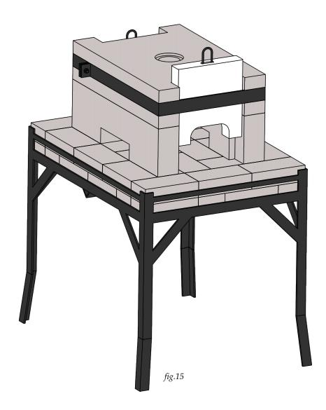
To make your door system functional you will need to install a pulley system, using a section of light cable attached to the door lifting ring. Perhaps you could set a number of small holes along the edge of the door and pin it at various heights useful to your production. For me, I prefer the free-lifting of the door and the ability to set it back on top of the heating metal to preserve temperature in the forge.
