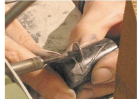
The images above and below were made using the copper wheel to grind and polish the grooves. The grit used was traditional emery in grades 200 and micro grit and finished with pumice.
