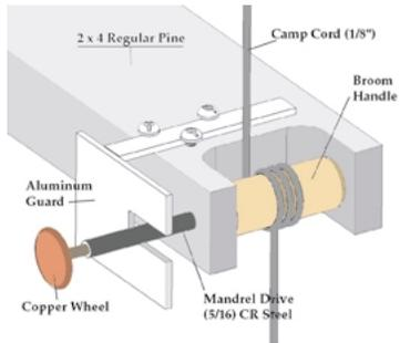
My lathe made with an old 2 x 4. In all it cost about \$1.00 and it works very well. The mandrel drive runs smoothly in the wooden bearings. The copper wheel is made with a penny and is set into the mandrel drive using wax. This is often called a Wax lathe. A small section of broom handle is used for the power drive which is also attached to the mandrel drive with wax. Very simple and it works.
