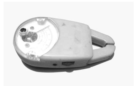
Fig. 21 The amp meter is an accurate and easy to use piece of shop equipment. By clamping around one of the insulated power leads you get a reading of amperes drawn.
