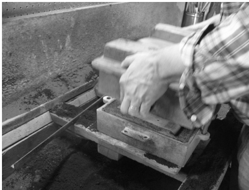
The mold halves are carefully separated.
