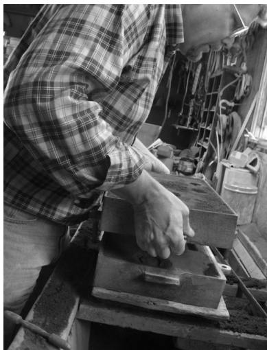
While using a careful touch the two parts of the mold are aligned using the pins and holes.
