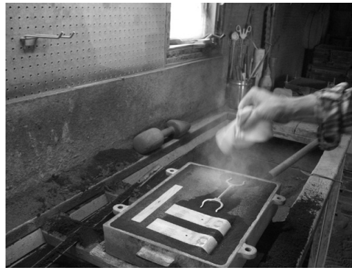
The DRAG mold is again dusted with talc.
