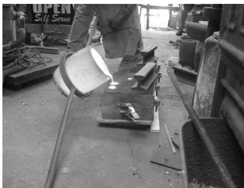
Here the mold is filled: notice the metal is showing in all three holes. That is good.
