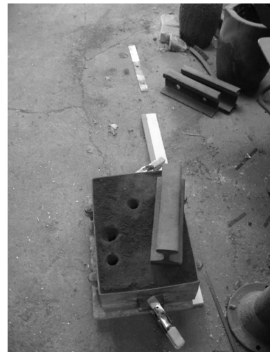
The setup is placed on the floor. Notice the clamps and weights. This is to keep the mold together during the pour so there will be no separation. Initially this might seem overly cautious but keep in mind the metal is heavy and can actually cause the top part of the mold to float if it were not secured as shown here.
