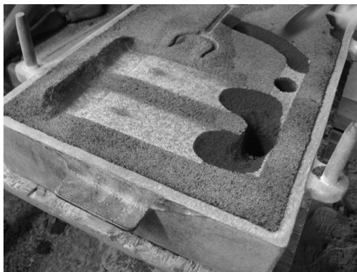
Using a tube cutter, Richard has punched a few holes into the COPE which will be the spew and vents.
