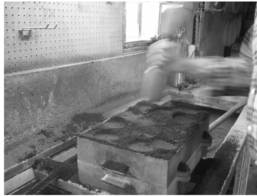
This COPE mold half is rammed with the maul.
