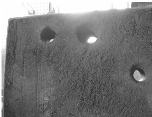
This is the very top side of the COPE and this shows the pouring basin and spew, the large hole in the middle. The other two holes are for venting.
