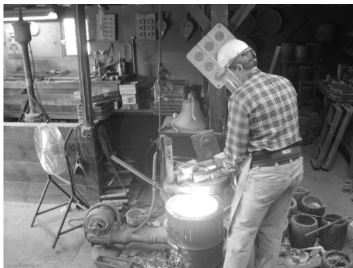
The furnace is opened and the crucible is removed.
